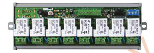
The 25ARO8 is an open frame heavy duty relay output module designed to withstand inductive load switching and high current applications removing the need to add extra contactors and heavy duty relays to control systems.
